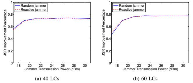
Fig. 7. The JSR improvement percentage for single jammer under different jammer transmission power with 40 and 60 local controllers, respectively.
