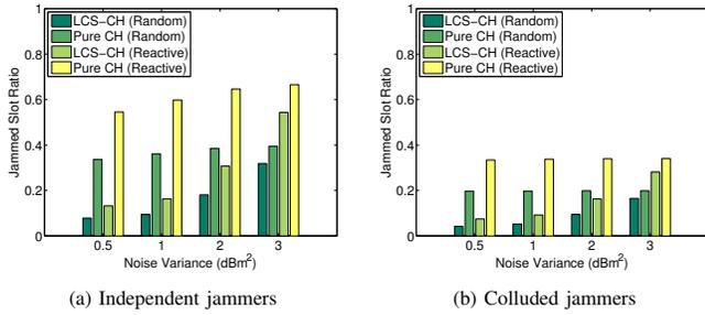
Fig. 6. Two jammers case: Comparison of JSR between LCS-CH and Pure CH with 40 local controllers.
