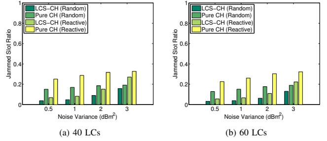
Fig. 5. Single jammer case: Comparison of Jammed Slot Ratio (JSR) between LCS-CH and Pure CH.
