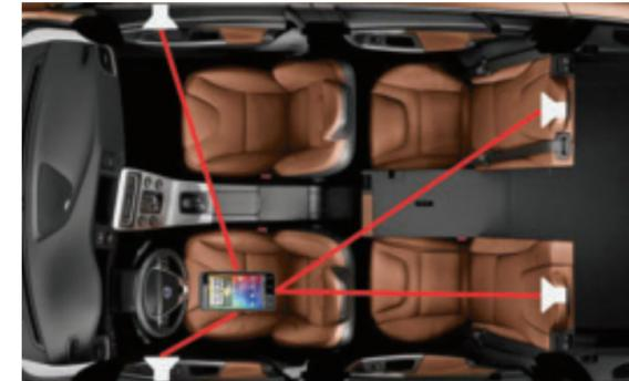
**Dr. Yingying Chen's detection system sends a series of customized, high-frequency beeps through an automobile's audio system to the speakers via smartphone, then uses acoustic ranging technology to determine which device belongs to the driver. The system is 90 to 95 percent accurate.**
