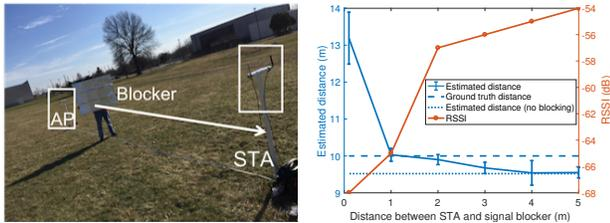
**Figure 6: Blocking LoS reception (1.4 m height, offset corrected).**
