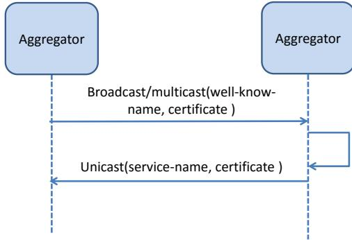
**Fig. 5:** General service discovery message flow for NDN and MF
