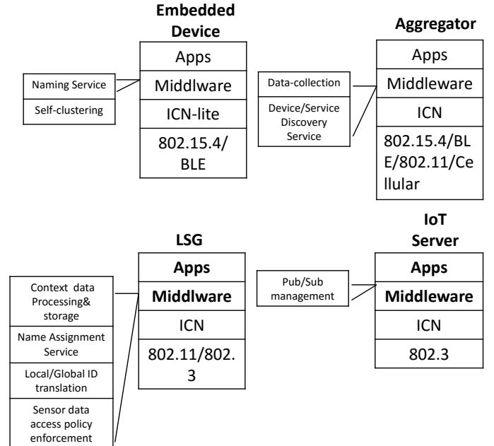
Fig. 4: System Architecture of ICN-IoT middleware
