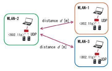
Figure 7. Experimental configuration for channnel assignment
