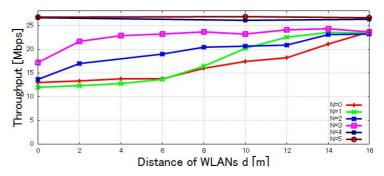
Figure 4. Distance and throughput in various channel distances(Planex router)
