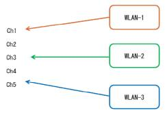
Figure 6. Image of channel assignment
