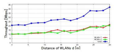
Figure 2. Throughput of co-channel m-WLANs as a function of distance
