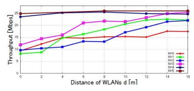
Figure 5. Distance and throughput in various channel distances(NEC router)
