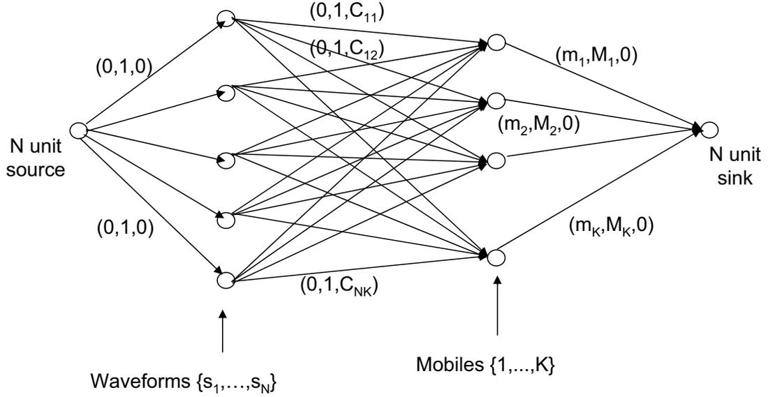
Figure 4.3: Flow network model for a Wireless system
