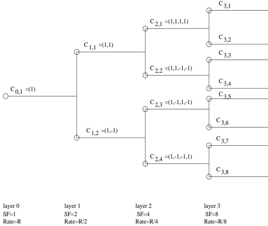
Figure 2.1: OVSF Code Tree.  $C_{i,j}$  represents node  $j$  on layer  $i$  and has a length of  $SF=2^i$
