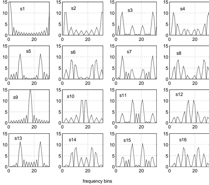
Figure 3.4: The Spreading Codes in Frequency Domain
