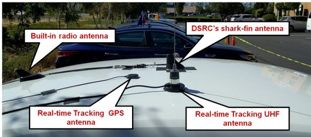
**Figure 2: Antenna setup on roof of test vehicles.**
