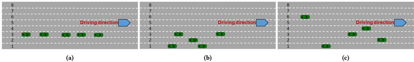
**Figure 4: The designed moving patterns for one group in the I-405 experiments: (a) five cars convoying; (b) five cars across different lanes; (c) five cars semi-randomly moving.**
