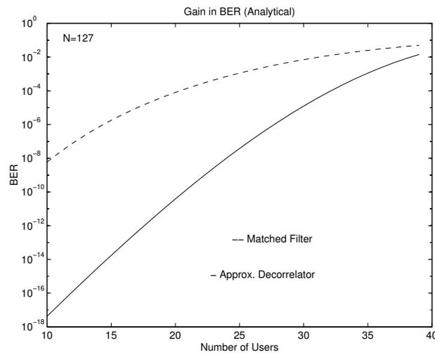
Fig. 6. BER gain  $P_k = P_1 = P$ , and  $P/\sigma_N = 20$  dB.
