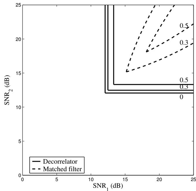
Fig. 4. SNR necessary to achieve  $\text{BER} \leq 3 \times 10^{-5}$  for both user. Shown for  $|\rho| = 0, 0.3, 0.5$ , and compared with the single-user matched filter detector regions.
