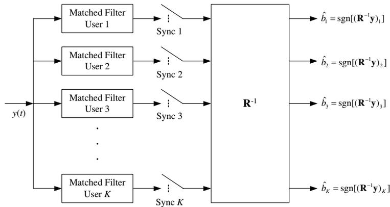
Fig. 1. Decorrelating detector for the synchronous channel.
