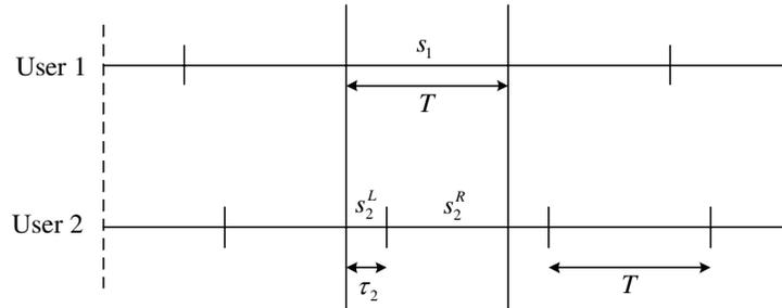
Fig. 3. Asynchronous two-user channel.
