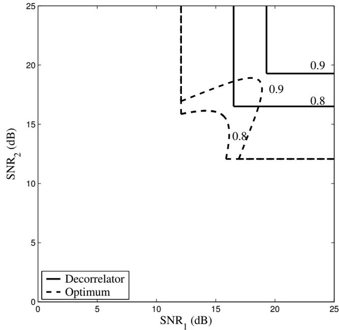
Fig. 5. SNR necessary to achieve  $\text{BER} \leq 3 \times 10^{-5}$  for both user. Shown for  $|\rho| = 0.8, 0.9$ , and compared with the optimal regions.
