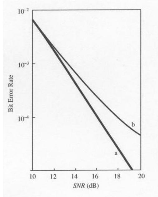
Fig. 4. Bit-error-rate of the single-user matched filter with 10 equal-energy users and identical cross-correlations  $\rho_{kl} = 0.08$ ; (a) exact, (b) Gaussian approximation.
