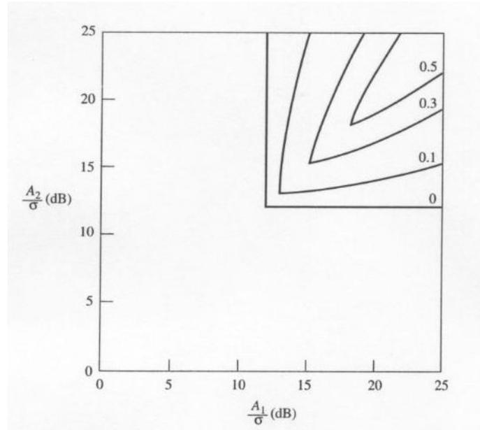
Fig. 2. Signal-to-noise ratios necessary to achieve bit-error-rate not higher than  $3 \times 10^{-5}$  for both users, parameterized by  $\rho$ .
