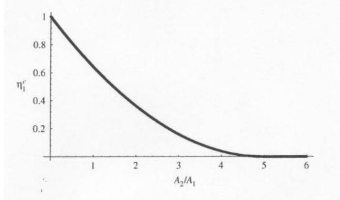
Fig. 6. Asymptotic multiuser efficiency of conventional detector as a function of the amplitude of the interferer;  $\rho = 0.2$  (linear plot).
