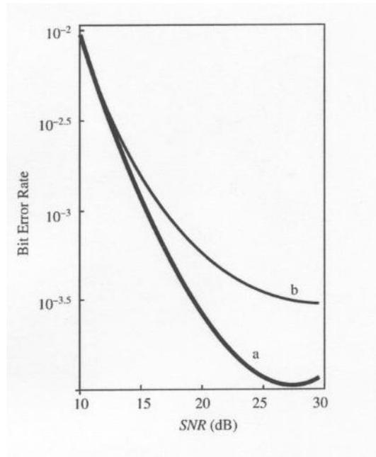
Fig. 5. Bit-error-rate of the single-user matched filter with 14 equal-energy users and identical cross-correlations  $\rho_{kl} = 0.08$ ; (a) exact, (b) Gaussian approximation.
