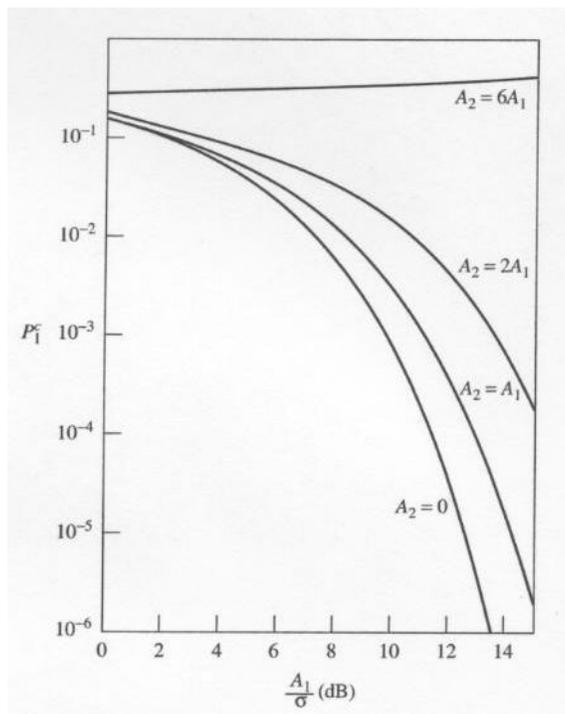
Fig. 1. Bit-error-rate of conventional detector with two synchronous users and  $\rho = 0.2$
