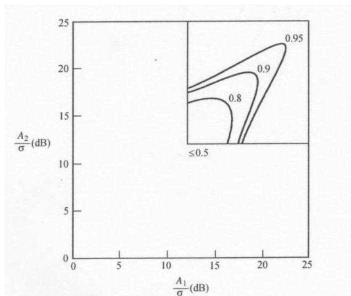
Fig. 8. Signal-to-noise ratios necessary to achieve optimum bit-error-rate not higher than  $3 \times 10^{-5}$  for both users.
