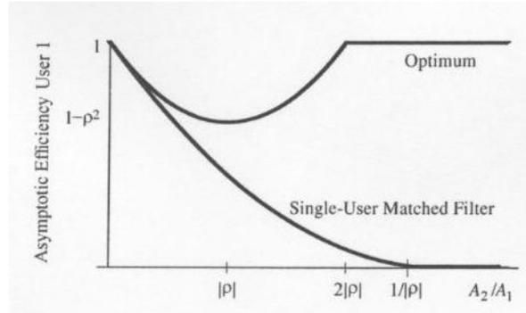
Fig. 7. Optimum and single-user asymptotic multiuser efficiencies for two synchronous users.
