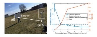
Figure 6: Blocking LoS reception (1.4 m height, offset corrected).
