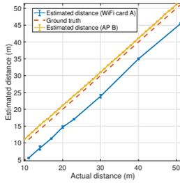
**Figure 4: Outdoor open space grass ground (0.7 m height). Comparing ranging results for using WiFi card A as AP compared to AP B while using WiFi card A as STA in both scenarios.**
