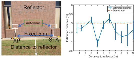
**Figure 7: Outdoor parallel to 7-floor building (1.4 m height, offset corrected).**
