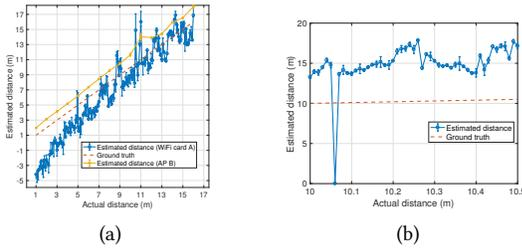
**Figure 10: (a) Indoor scenario (room (0.7 m height)) for comparing ranging results for using WiFi card A as AP compared to AP B while using WiFi card A as STA in both scenarios. (b) 1 cm step in indoor room (1.4 m height, offset corrected). Zero distance represents no signal.**
