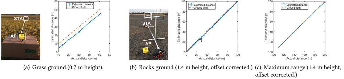
**Figure 3: Outdoor open space. This setup uses the WiFi card A for both STA and AP sides.**
