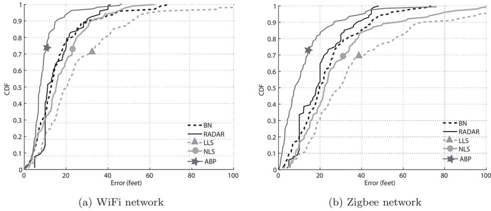
Figure 12.3: Performance comparison: localization error CDF across different algorithms under the WINALB experimental scenario [27].
