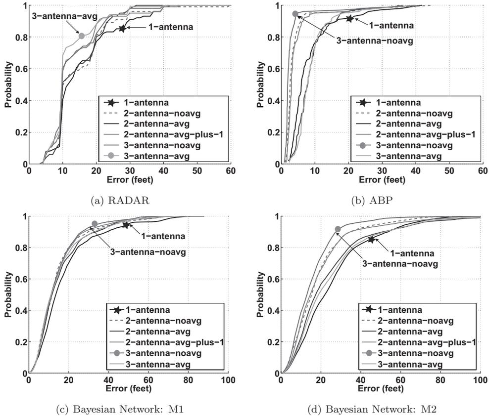
Figure 12.6: Localization error CDFs when using multiple antennas in the WINLAB experimental scenario under the WiFi network [27].
