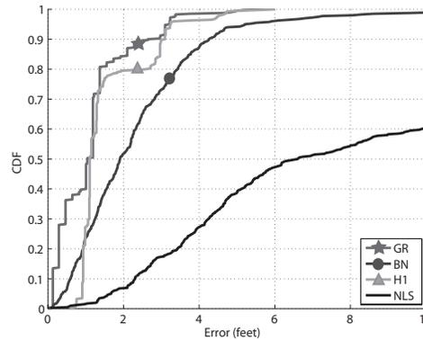
Figure 12.4: Performance comparison: localization error CDF across different algorithms under the ORBIT testbed experimental scenario [28].
