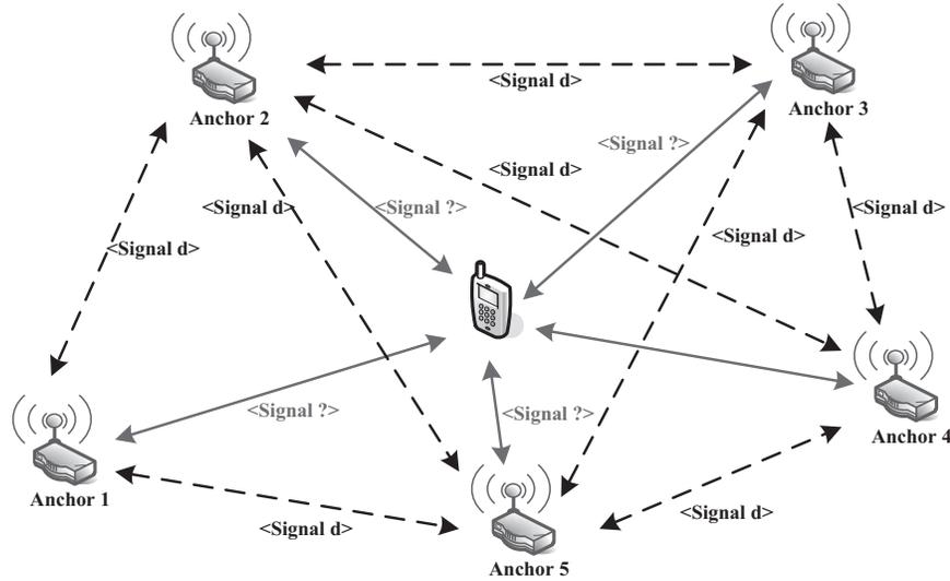
Figure 12.5: System architecture for real-time infrastructure calibration.
