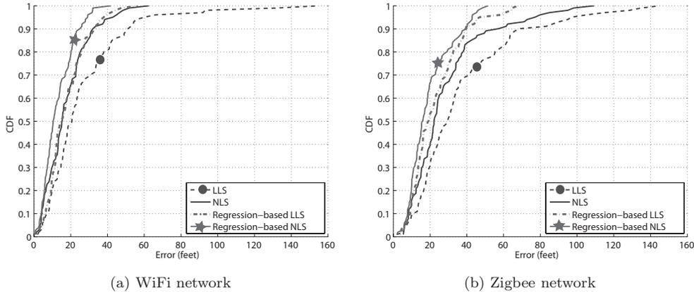
Figure 12.7: Regression-based approach: localization error CDFs in two networks [14].
