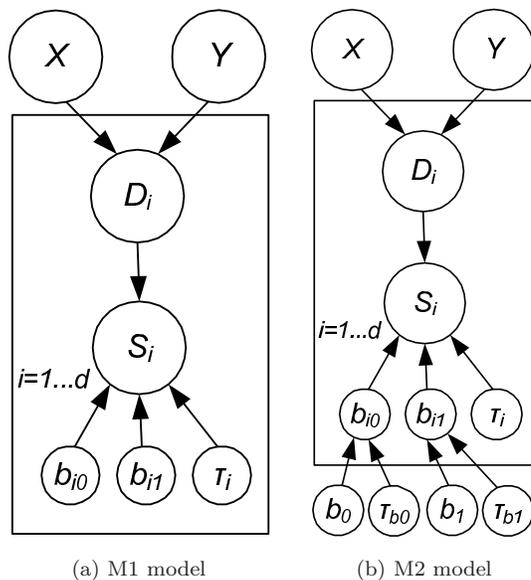
Figure 12.1: Bayesian Networks localization algorithm: Bayesian Graphical Models using plate notation
