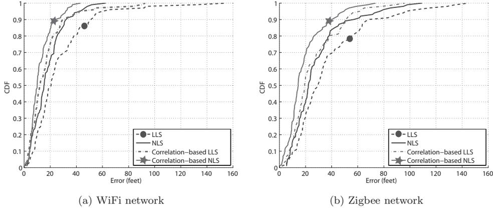
Figure 12.8: Correlation-based method: localization error CDFs in two networks [14].
