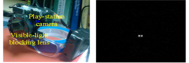
Contraction of an IR-Camera with our smart-glass receiver Image output of the IR camera (white blobs correspond to light output from a tag)
