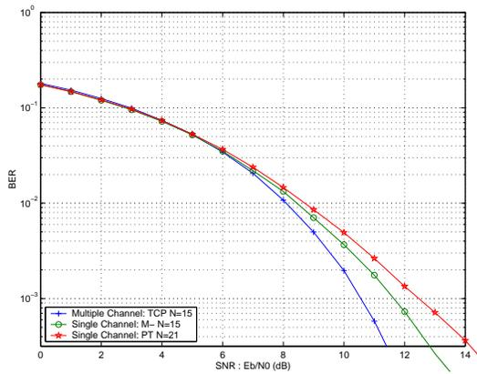
Fig. 1. Single User: Parallel channel UWB system with TCP versus Single channel UWB system with m- and perfect ternary sequence
