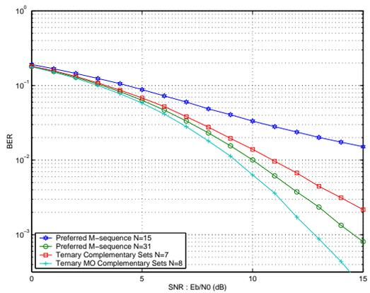
Fig. 2. Two Users: Parallel channel UWB system with ternary complementary sets versus Single channel UWB system with preferred m-sequences
