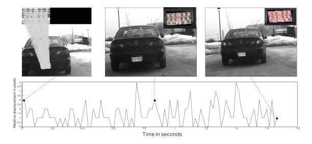
Figure 4: Left: SIFT feature-based recognition showing corresponding features between the LED template and the query image. Center and Right: LK tracking of an LED Transmitter. The inset shows a magnified view of the tracked LEDs as indicated by the white crosses. Bottom: Relative displacement of an LED due to the motion of the car over 120 frames.
