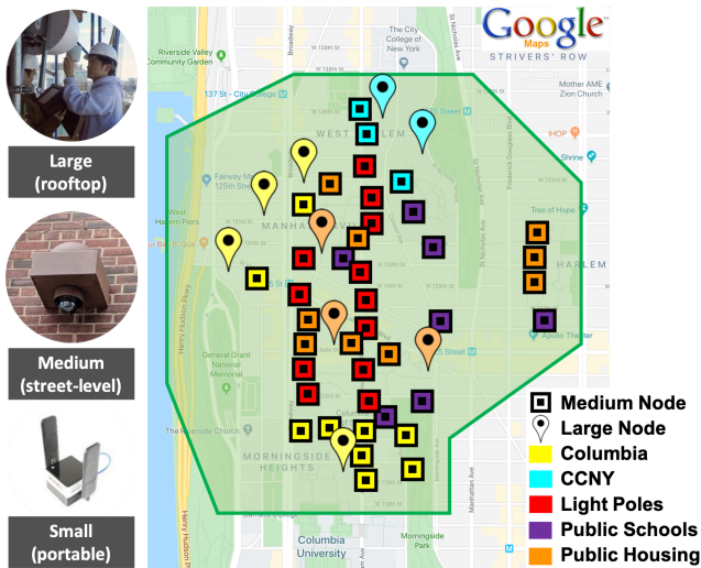
Figure 10: COSMOS' envisioned deployment area of about 1 sq. mile covering about 15 city blocks and about 5 city avenues, with tentative deployment sites marked on the map (see also Fig. 2 for the network connectivity and the three deployment phases).
