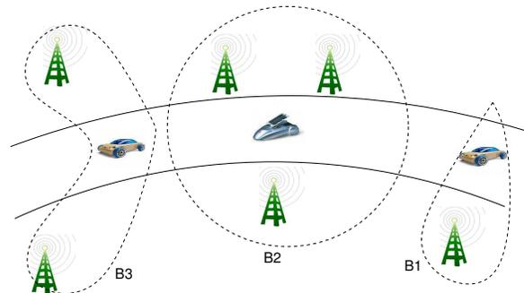
Figure 1: Different beam configurations for communication between clients and the receivers. B1 uses directionality with a single receiver, B2 uses diversity with all visible receivers, and B3 uses a combination of directionality and diversity with a subset of the visible receivers.
