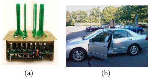
**Figure 8: (a) Transmitter with beamforming antenna, (b) Transmitter enclosed in a box and mounted on a car.**
