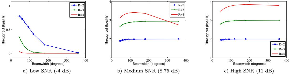
**Figure 3: Tradeoff Illustration.** Throughput is maximized at a specific combination of rate and beamwidth, and individually controlling either the beamwidth or the rate leads to local maximas (making the case for joint adaptation).
