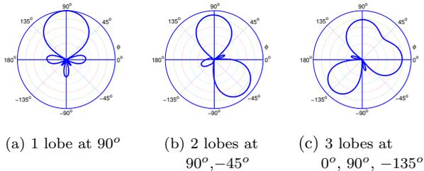
Figure 5: Example beams with different number of main lobes at different angles. The motion of the car is along zero degrees.
