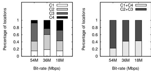
**Figure 2: A combination of directionality and diversity (C2 or C3) achieves lower PER at a majority of locations relative to vanilla directionality (C1) and diversity (C4). C1, C2, C3, and C4 correspond to reception using 1, 2, 3 and 4 receivers respectively.**
