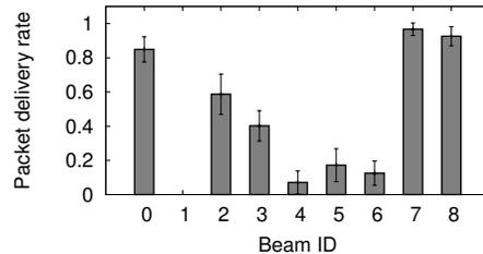
**Figure 20: Angular Localization. Cost of choosing the “wrong” beam is high. Beam ID 0 = Omni.**
