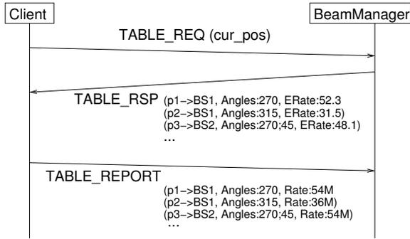
**Figure 7: Protocol Overview.**  $p_1$ ,  $p_2$ ,  $p_3$  represent GPS locations, and BS1, BS2 represent the anchor base stations. We define a GPS location (area) by considering only the first four digits after the decimal of the latitude and the longitude.
