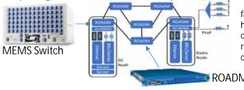
fast front-haul/midhaul/back-haul connectivity between radio nodes and edge cloud
