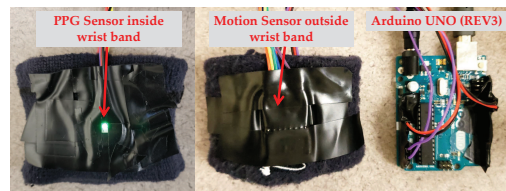
Fig. 9. Prototype: wrist-worn PPG sensing platform.
