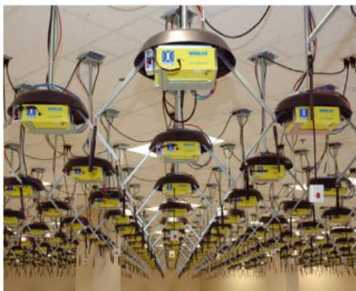
(a) Wireless nodes lay out in ORBIT testbed
