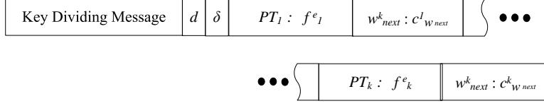
Fig. 5: Packet format of key dividing message
