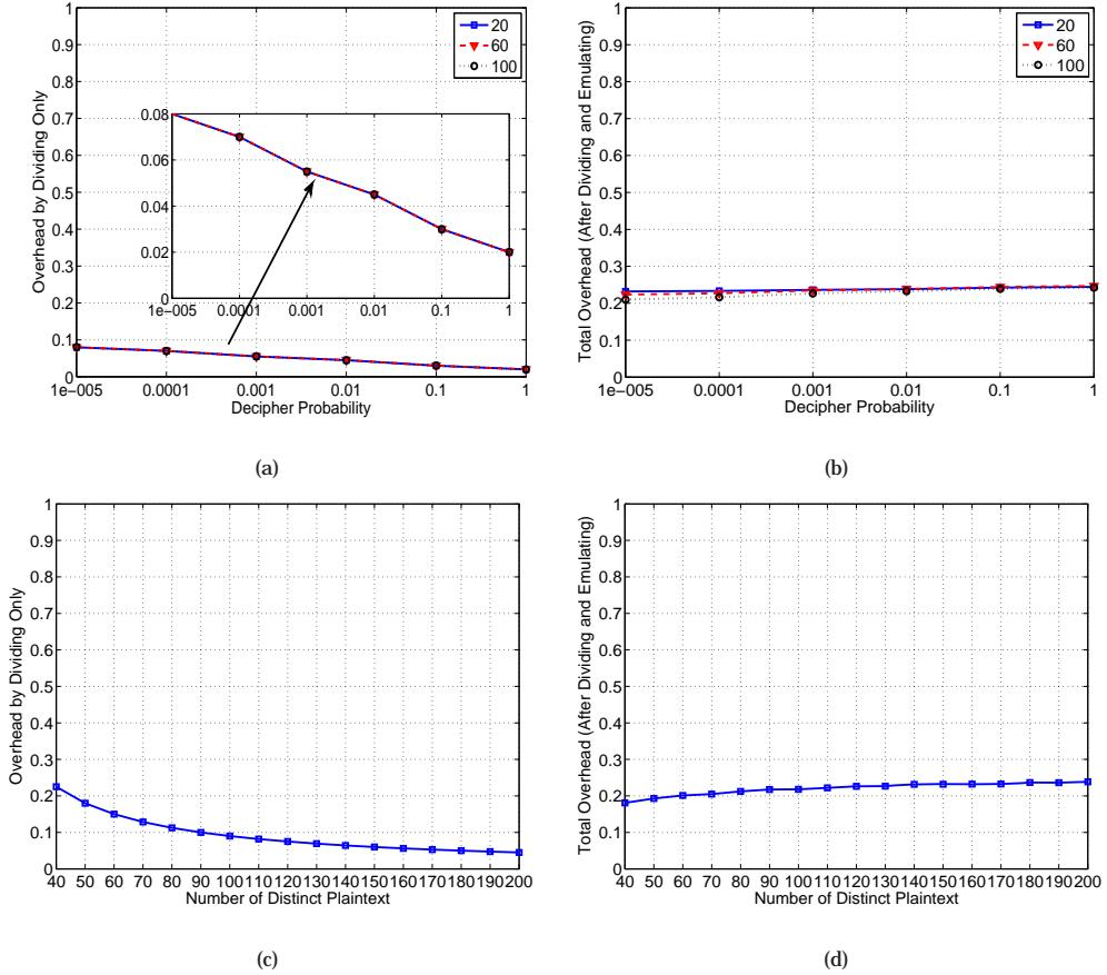
Fig. 3: Overhead of Dividing and Emulating when coping with the global frequency-based attack: (a) and (b) show the overhead by dividing and emulating under various decipher probability and network sizes  $N = 20, 60$  and  $100$ , with the number of distinct plaintext values fixed as  $200$ ; (c) and (d) present the overhead by dividing and emulating under various distinct plaintext values with the decipher probability fixed as  $0.01$ .
