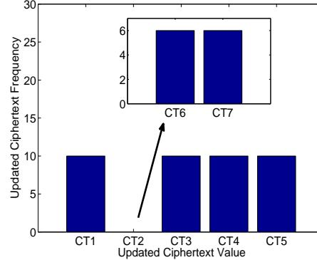
Fig. 12: Distribution of ciphertext values by dual encryption method after updates
