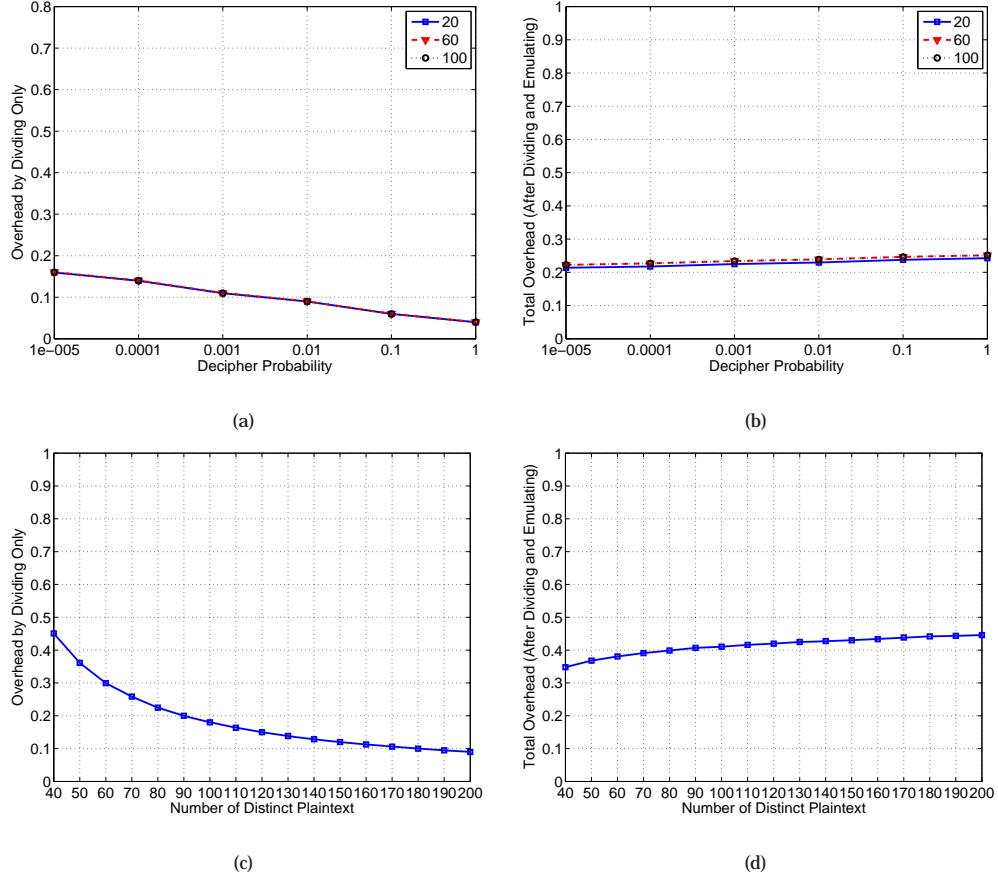
Fig. 2: Overhead of Diving & Emulating when coping with local frequency-based attack with network size  $N = 20, 60$  and  $100$ : (a) and (b) measures the overhead by dividing and emulating under various decipher probability, with the number of distinct plaintext values fixed at 200; (c) and (d) shows the overhead by dividing and emulating under various distinct plaintext values, with the decipher probability fixed as 0.01 and network size fixed as 60.
