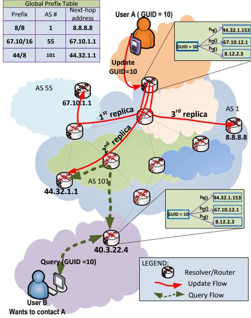
Fig. 2. DMap with K=3 independent hash functions
