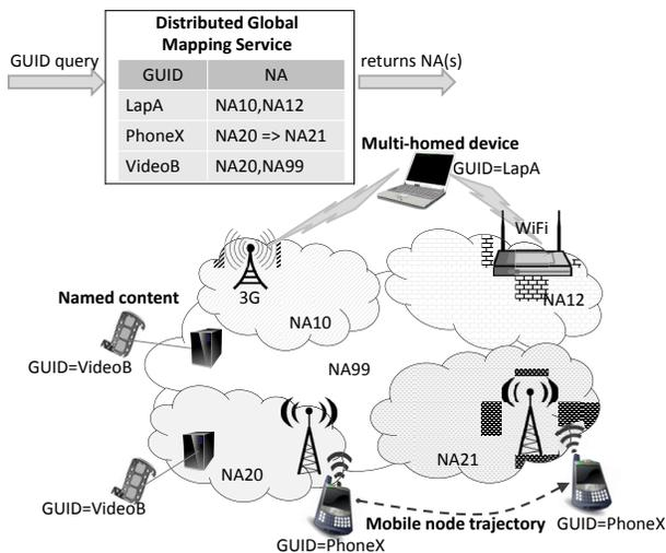
Fig. 1. Distributed global identifier to locator mapping service
