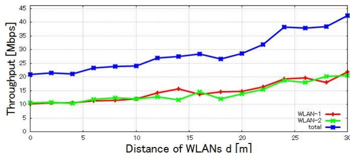
Figure 2. Throughput of co-channel m-WLANs as a function of distance
