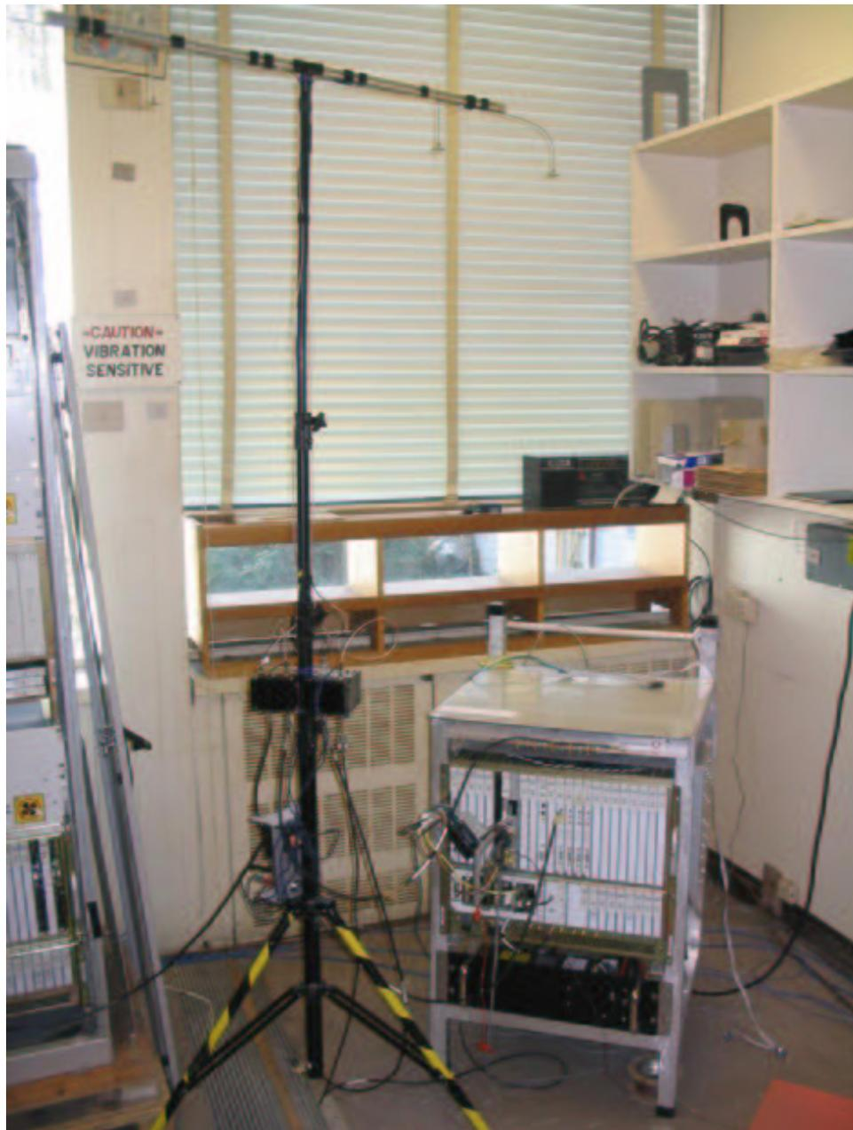
Figure 1: Multi-antenna base station.
