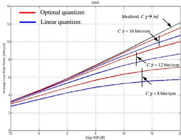
Figure 5: Uplink zero-forcing 8x8, optimal and linear quantizer.
