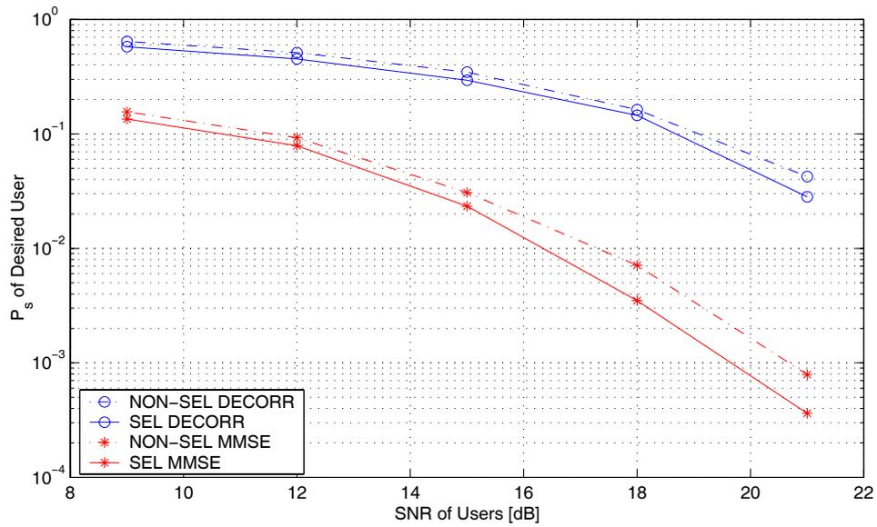
Figure 4: Comparison of selective and non-selective detectors. The upper graph shows the performance of a lightly loaded system with  $(K, M, N) = (2, 4, 20)$ , whereas the lower graph is for a fully loaded system with  $(K, M, N) = (5, 4, 20)$ .
