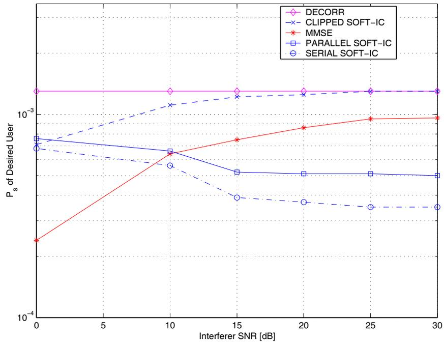
Figure 3: Comparison of soft-ICs in near-far scenario with  $(K, M, N)=(2, 4, 20)$ . Desired user's SNR= 14dB.
