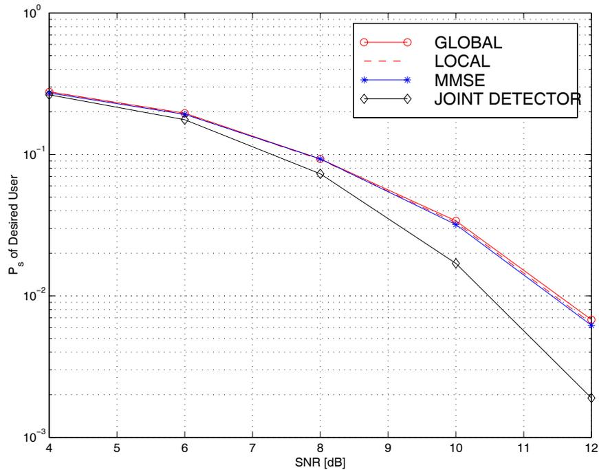
Figure 1: Comparison of various noncoherent detectors with  $(K, M, N)=(2, 4, 20)$ .
