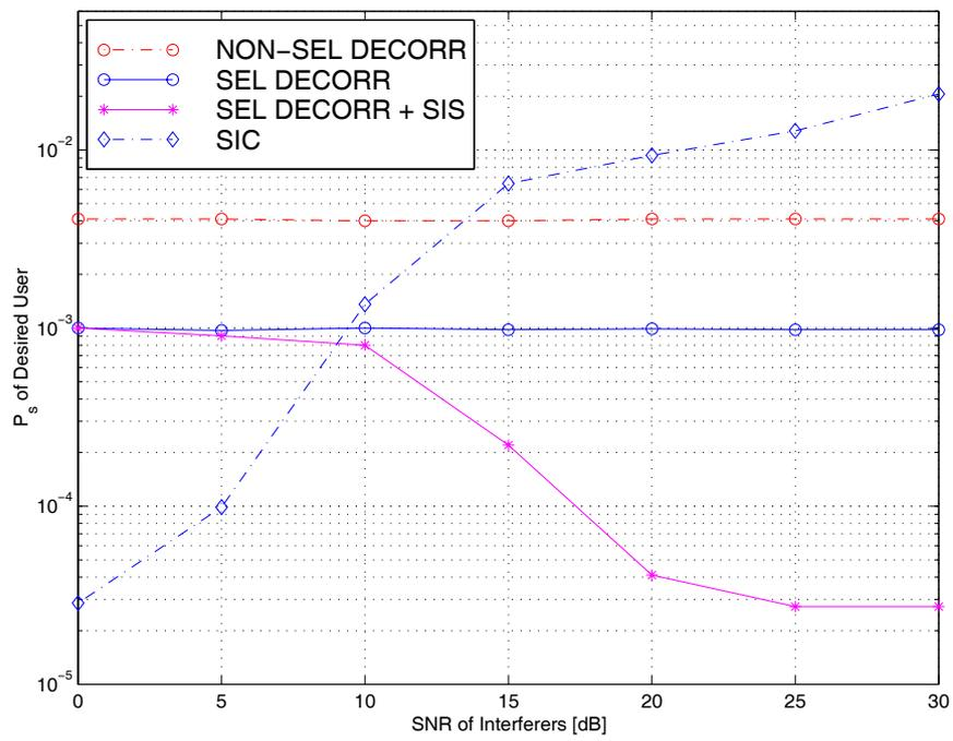
Figure 7: Performance of selective decorrelator with SIS with  $(K, M, N)=(3, 4, 20)$  and desired user's SNR at 15dB.
