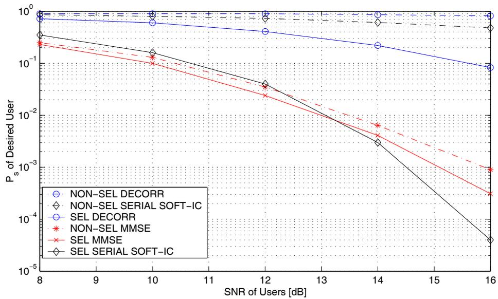
Figure 5: Comparison of selective and non-selective detectors with higher processing gain  $N = 64$ . The top figure represents a moderately loaded system with  $(K, M, N) = (4, 8, 64)$  whereas the bottom figure represents a fully loaded system with  $(K, M, N) = (4, 16, 64)$ .
