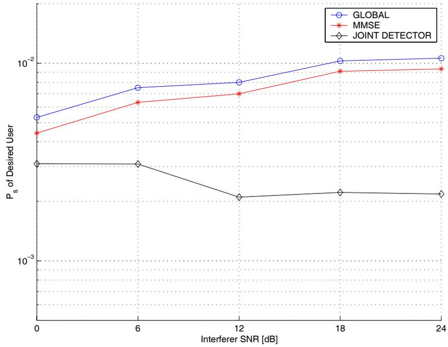
Figure 2: Performance in the near-far scenario with  $(K, M, N)=(2, 4, 20)$ . Desired user's SNR= 12dB.
