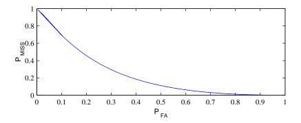
After all of this work, we see that the sensor is not particularly good in the the ense that no matter how we choose the thresholds, we cannot reduce both the miss and false alarm probabilities under 30 percent.
