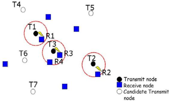
Fig. 2. A network populated with candidate transmit nodes and receive nodes. A candidate transmit node attempts a transmission if there are receive nodes in its transmit range.
