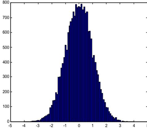
Figure 2: MATLAB plot of frequency distribution (histogram) of random variables generated by the Box–Muller method. The abscissa represents the value of the random variable and the ordinate represents the number of corresponding occurrences.
