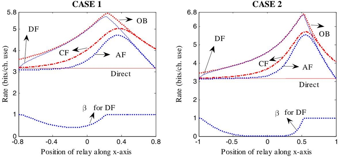
Figure 3: Sum rates for no fading GMARC with  $P_1 = P_2 = P_3 = 6$  dB and  $\gamma = 4$
