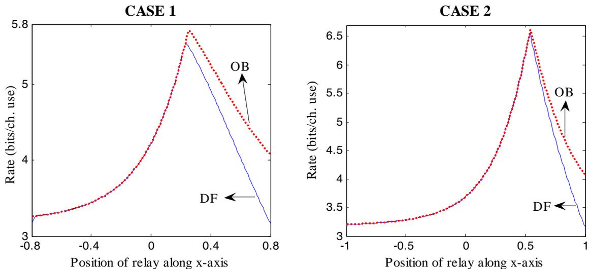
Figure 4: Sum rates for ergodic phase-fading GMARC with  $P_1 = P_2 = P_3 = 6$  dB and  $\gamma = 4$
