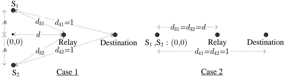
Figure 2: Two geometries for the two-source Gaussian MARC
