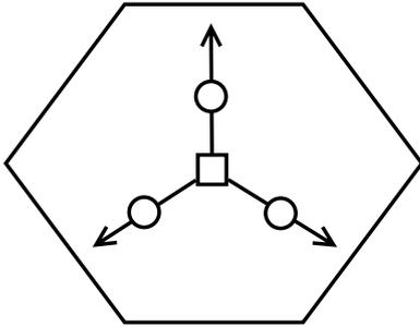
Fig. 3. Position of relay location in a cell. The relays (represented by small circles) are placed at half the cell radius in the direction (given by the arrows) of the main lobe of the sector antenna. The base station at the center of the cell is represented by a square.
