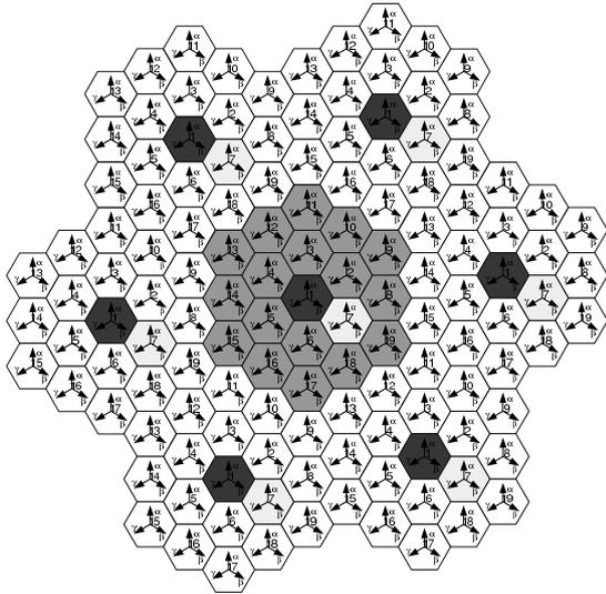
Fig. 1. Wrap-around simulation model. The center ring of 19 cells are used for the simulation. The surrounding cell activity is mirrored in the center ring. The direction of the arrows represent the direction of the main lobe of the sectorized antenna.
