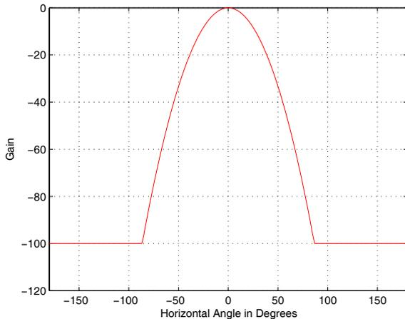
Fig. 2. Antenna gain pattern (from [18]) as a function of the horizontal angle in degrees. The mathematical expression for the gain is given in equation (1).
