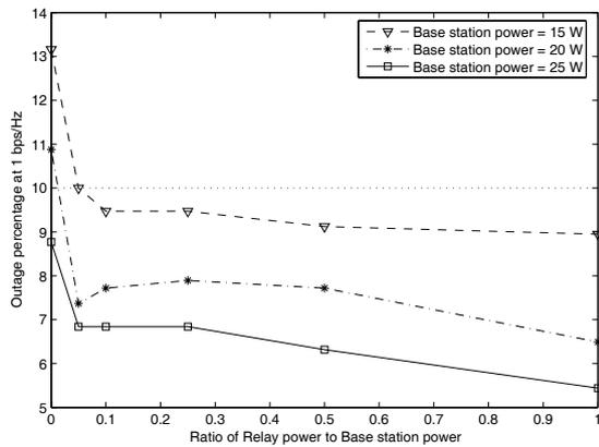
Fig. 4. Variation of outage with relay powers and base station powers. As we increase the base station powers with no relays in the system (ratio = 0), the outage decreases and saturates at around 5%, due to the interference limit. The interference limit sets in very quickly even for smaller values of relay powers.
