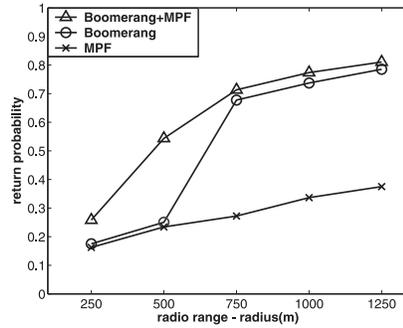
Fig. 8. Return probability when varying radio range values with  $T_{ho}$  of 1000 seconds
