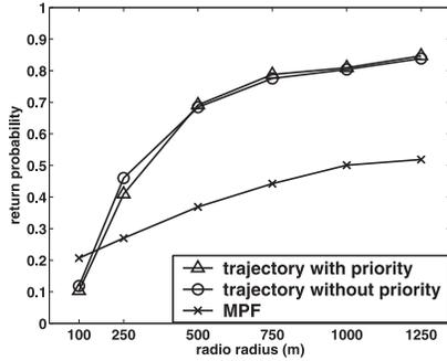
Fig. 7. The comparison of three anchoring schemes when increasing the radio range radius.  $T_{ho} = 750$  seconds.
