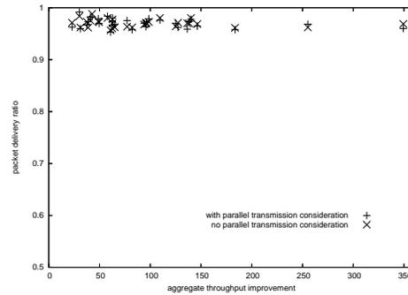
**Figure 10: Improvement in aggregate throughput with parallel transmission consideration; in most experiments, parallel transmission can admit 50 – 150kbps more traffic without a noticeable reduction in PDR.**
