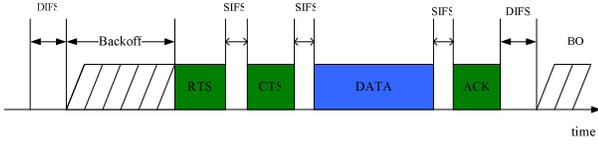
**Figure 1: Operation of Four-Way Handshake in the 802.11 DCF**
