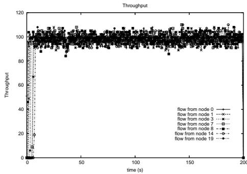
**Figure 7:** In the network with 20 randomly positioned nodes, only 7 (out of 9) flows are admitted; the 7 admitted flows achieve their desired throughput
