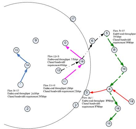
**Figure 9: Example of parallel transmissions, only when considering overlap due to parallel transmissions, flow 1 – 14 – 13 can be admitted**
