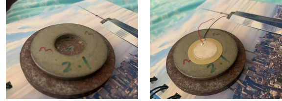
(a) Metal disc used to secure the rim of the piezo, allowing flexing. (b) Metal disc with piezo fixed.
