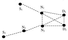
Figure 1: Using omni-directional antenna Low Priority Flow (S<sub>2</sub>-D<sub>2</sub>) is disturbing High Priority Flow (S<sub>1</sub>-D<sub>1</sub>). Dotted Lines show omni-directional connectivity
