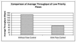
Figure 6: Comparison of Average Throughput of Low Priority Flows
