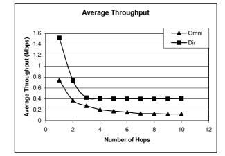
Figure 4. Comparison of AverageThroughput of two flows using Directional and Omni-directional Antenna with increasing number of hops
