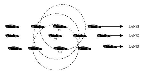
Figure 1(a). Overlapping transmission-zones of cars C1, C2 and C3 using omni-directional antenna inhibits the possibility of simultaneous communication among the vehicles along the lanes 1, 2 and 3
