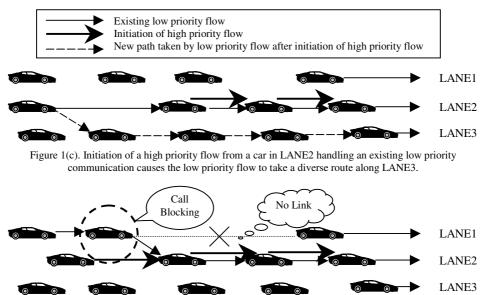
Figure 1(d). Initiation of a high priority flow from a car in LANE2 handling an existing low priority communication forces the low priority flow to block itself due to the absence of any other alternative path
