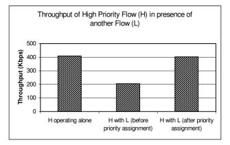
Figure 5. Throughput of a High Priority Flow (H) in presence of another Flow (L) with and without Priority Scheme
