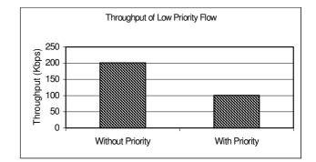
Figure 6. Throughput of a Low Priority Flow in presence of another Flow with and without Priority Scheme
