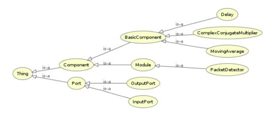
Figure 2: Classes in the Packet Detector ontology
