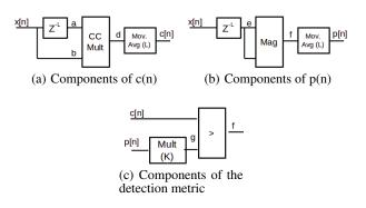
Figure 1: Components derived from packet detection unit
