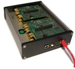
Figure 1: CRKIT hardware platform with enclosure, dual WDRs mounted on baseband processor.
