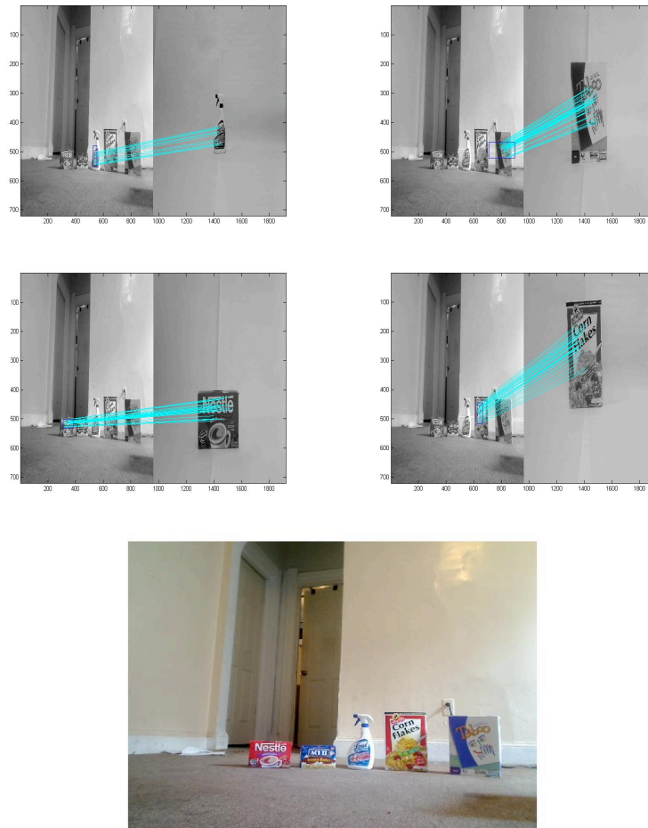
Figure 3: These images show our first task of the robot, which is to find all of the objects in the scene that match objects in our codebook. As you can see the program cycles through the scene and compares it to each of the images of our objects located in the codebook. If enough point correspondences are found then the program outputs a list of all the objects that it found.
