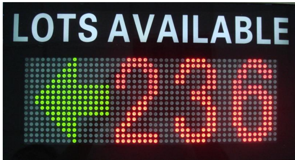
Fig. 2. Example of display showing number of spots available on a specific parking garage floor
