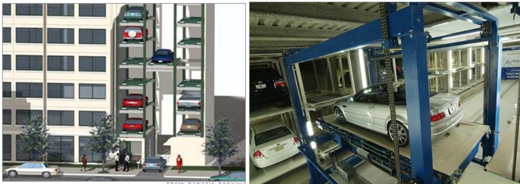
Fig. 1. Computer generated model of a robotic parking structure (left) and a real world example of one such system (right)
