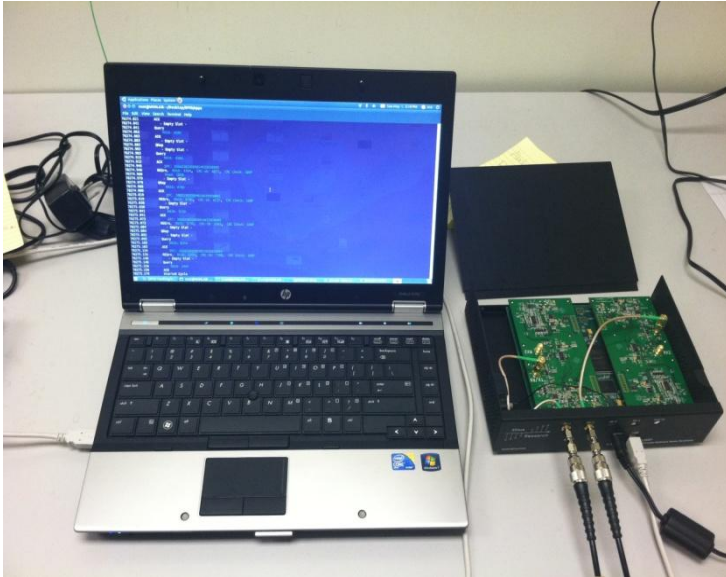
Fig. 20: USRP and Laptop with GNU Radio stands
