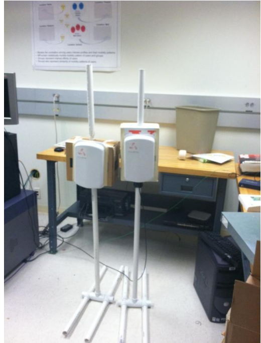
Fig. 21: 2 Alien Antennas on stands
