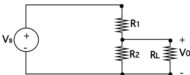
**Fig. 3 A Voltage Divider Connected To A Load Of  $R_L$  ohms**
