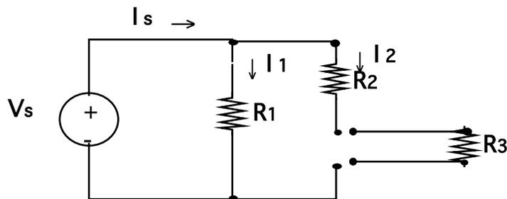
**Fig. 7 A Current Divider Circuit**
