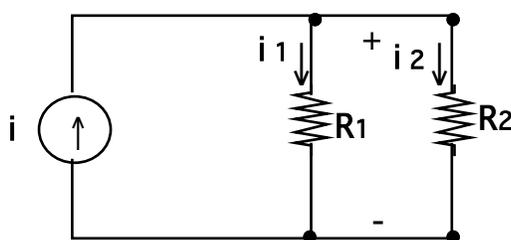
**Fig. 4 A current Divider Circuit**
