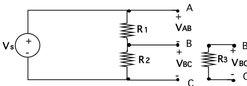
**Fig. 6 A Voltage Divider Circuit**
