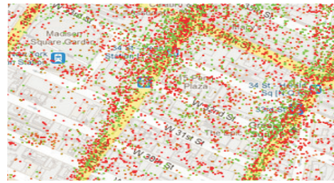
Fig. 5. Estimated Wi-Fi AP locations in a 0.4x0.5 sq.mile area in Manhattan, NY. Red dots indicate single citation in the crowd sourced war-driving database. Green dots indicate multiple citations. Source:WiGLE [9]
