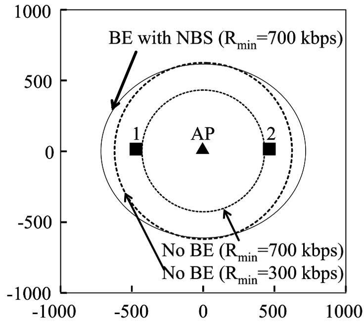
Fig. 6. Improvement in coverage and rate in a  $2000 \times 2000$  m<sup>2</sup> region.
