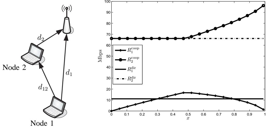
Fig. 1. Bandwidth exchange enhances rates for both nodes simultaneously with  $d_1 = 400$  m,  $d_2 = 150$  m,  $d_{12} = 300$  m,  $\kappa = 6 \times 10^6$  MHz  $\cdot$  m<sup>3</sup>/mW.
