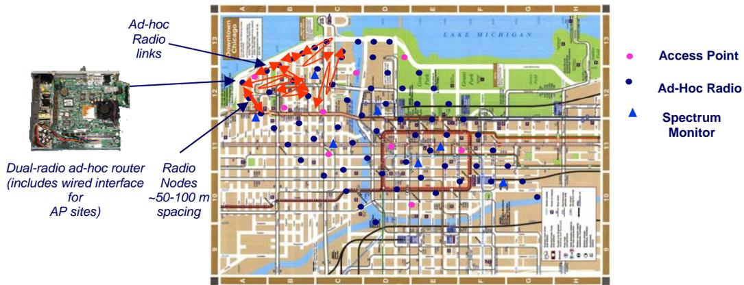
Figure 13 Deployment Concept for Ad-Hoc Mesh Network
