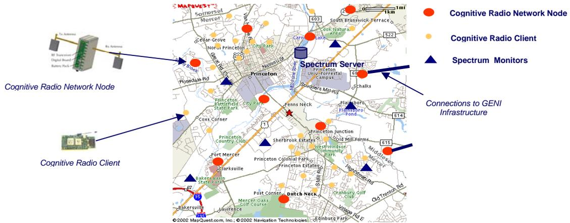
Figure 16 Deployment Concept for Cognitive Radio Demonstrator Network
