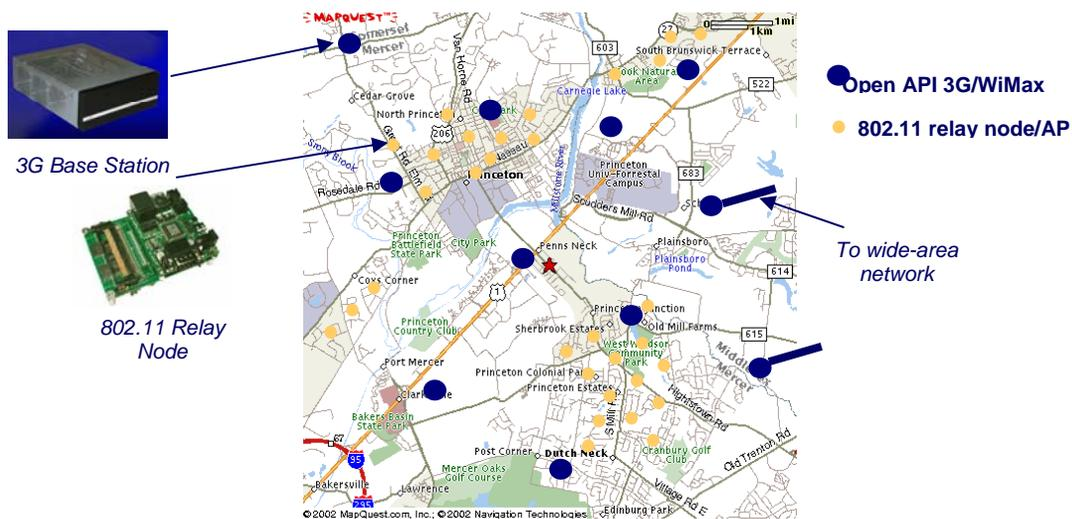
Figure 14 Deployment Concept for Open API Wide-Area Wireless Network
