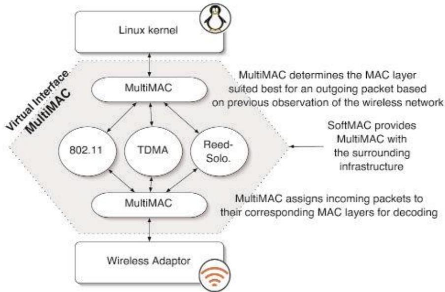
Fig 7. Architecture for virtualization of wireless MAC layer
