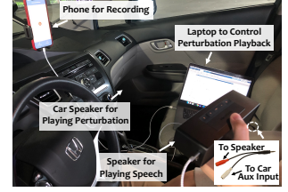
Figure 8: Illustration of the inside-vehicle setup.
