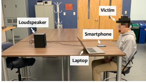
Figure 9: Illustration of the live human speech setup.
