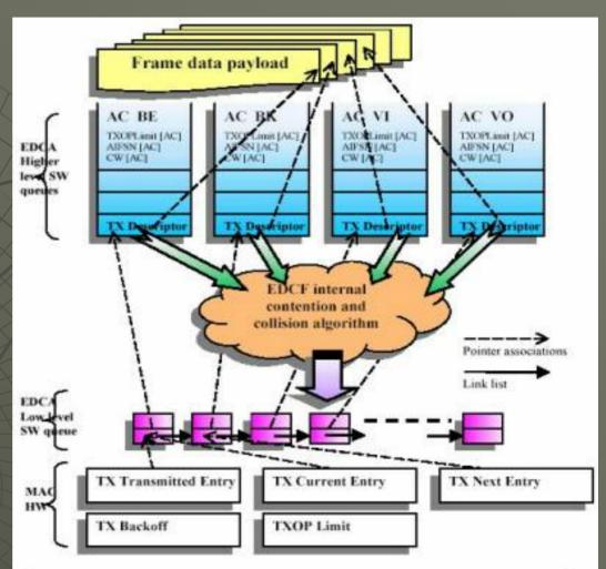
The frame data payload is stored in a pool of buffers in RAM
