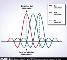
FIGURE 4: Orthogonality in an OFDM system occurs when at the peak of each subcarrier spectrum, the contribution from all other subcarriers is zero.
