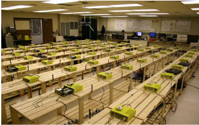
Figure 1 Prototype 8x8 ORBIT radio grid
