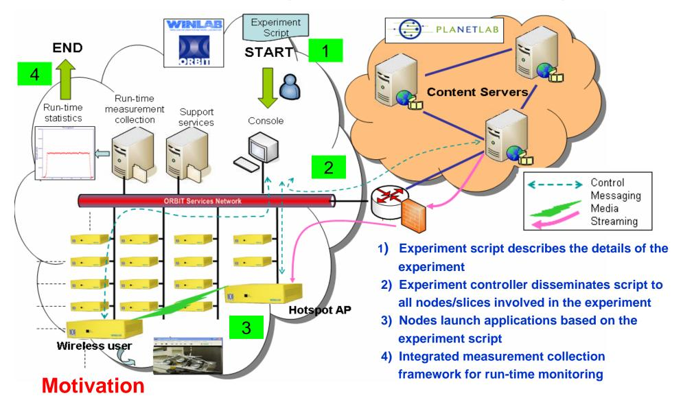
Federate wired and wireless testbeds to enable end-to-end experiments involving heterogeneous networks
