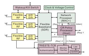
Fig. 4. A generic SDR/CR platform involving RF processors, baseband processor, network processor, and the cognitive radio processor. Note that TRIESTE regulates via a TCB component and an externally-accessible authenticated kill-switch.
