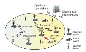
Fig. 1. TRIESTE Architecture is composed of multiple tiers of actors: lowest tier are the cognitive radios, above that will be the DSA-tier (Distributed Spectrum Authority), and above that are the Spectrum Law Makers (aka. FCC).
