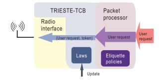
Fig. 2. The architecture of the Cognitive Radio with on-board TRIESTE-TCB.
